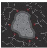
Binder modified with cross-linked polymer cannot diffuse, leaving the RAP binder unmodified.
