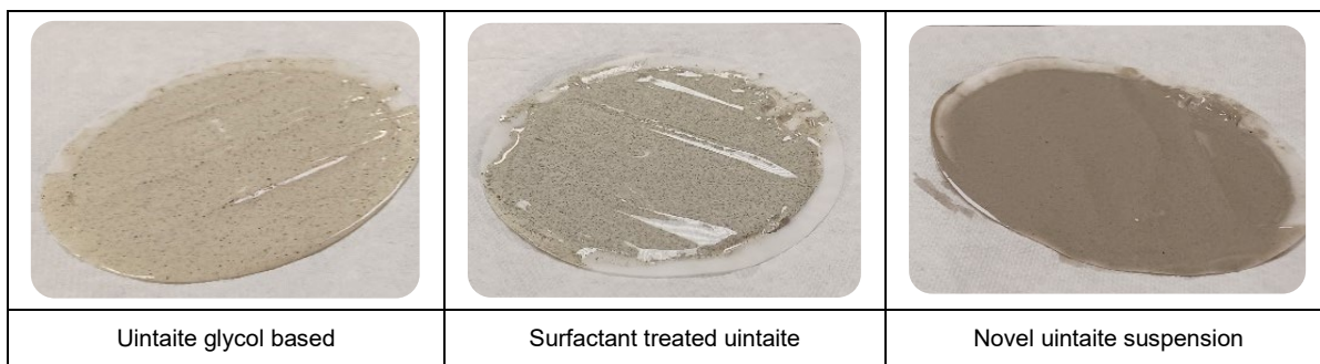
Figure 12. Filter cakes photos after the API fluid loss test
